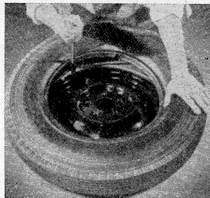
FIG. 15.—Final fitting of one bead with a lever.
