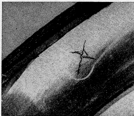
FIG. 5.—A severe impact has fractured this casing.
