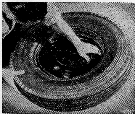
FIG. 14.—Fitting the cover. Note that the bead is pressed well into rim.
