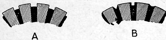
FIG. 5.—Method of undercutting the commutator insulation.
